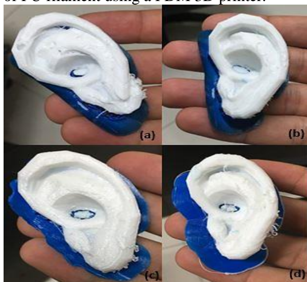
Fig. 2: TPU auricle samples achieved at several polymer filament's infill rates. (a) 25%, (b) 50%, (c) 75%, and (d) 100%.
